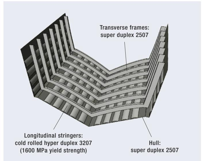
➤ The stringers are spot welded to the hull plates. The frames, welded to the stringers, are not in direct contact with the hull. The flexibility of the stringers allows them to absorb the wave force preventing the hull from bucking.
