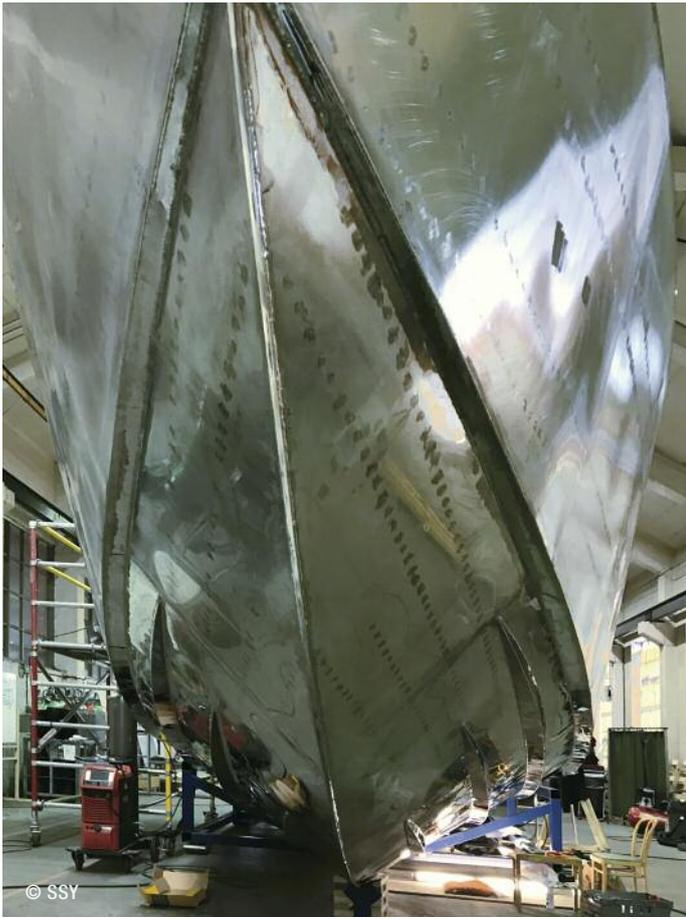
› Stainless steel hull of a prototype at the ship yard before mirror-polishing under the waterline and painting above it.
